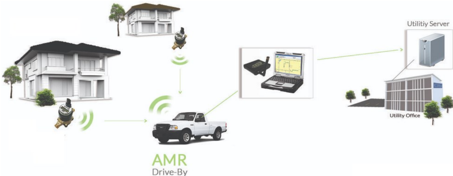
Pictured below: Illustration showing the Automatic Meter Reading (AMR) process
