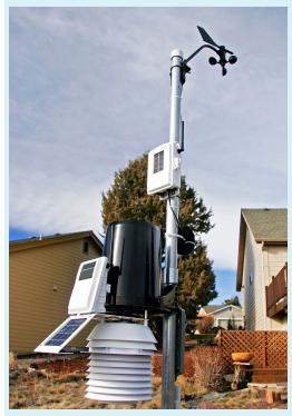
Byrum's equipment (pictured above) measures wind speed and direction, rainfall, barometric pressure, temperature, humidity, and more. View data at www.seesthewind.com
